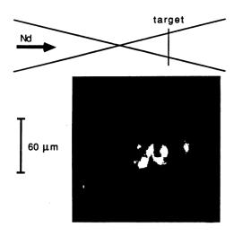
Fig. 1. Cross section of the interaction region imaged by the second harmonic light emitted forward. The image was obtained with a gated image intensifier using a narrowband filter at 5320Å. The 120 ps gate-window was centered at the peak of the laser pulse. Target: 1. µm plastic foil. Target position: 0.5 mm behind the best focus. Nominal irradiance on target: 2 10<sup>13</sup> W/cm<sup>2</sup>. Filaments and related interference fringes are apparent.
