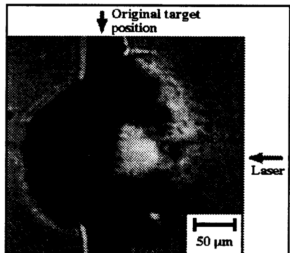
Fig. 3. Polarigram taken during the short pulse interaction with a preformed plasma in the same conditions of fig. 1.
