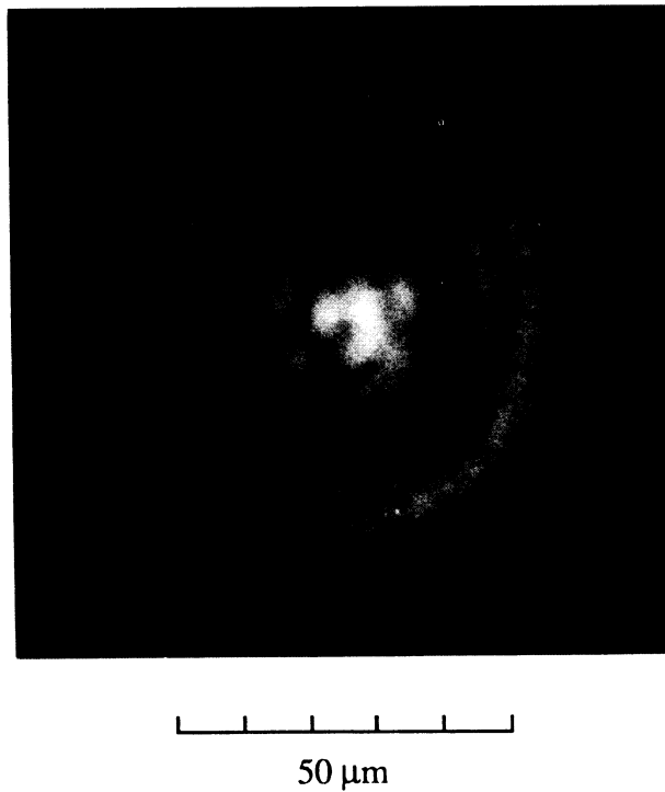
FIGURE 5. Image of SH sources taken with the target in the maximum SH power position: 120-ps gate at the peak of the laser pulse. Nominal intensity on target: 3 \times 10^{13} W/cm 2 .
