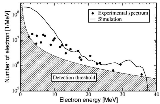
FIG. 4. Spectrum of the electrons in the collimated beam. Black dots represent the experimental data. Also shown is the detection threshold of the electron spectrometer. The solid line is the spectrum of the electrons in the collimated beam (within 3 deg around the axis in Fig. 3) as obtained from the PIC simulation.
