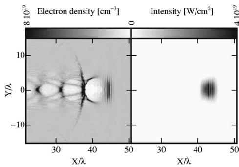
FIG. 5. 3D PIC simulation: electromagnetic field distribution of the laser pulse (right) and electron density distribution (left) at the time when the laser pulse ( $\lambda = 800$  nm) is going to leave the plasma. Clearly visible is the formation, in the wake of the pulse, of an electron wave of  $\lambda_p = 5.1 \times 10^{-4}$  cm.
