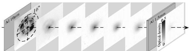
FIG. 2. Densitometer scans of the radiochromic films after exposure to the energetic electron beam produced by interaction of an ultraintense laser pulse with a preformed plasma located at 26 mm on the left. The angular scale is also shown for reference. The arrow indicates the electron beam propagation axis.
