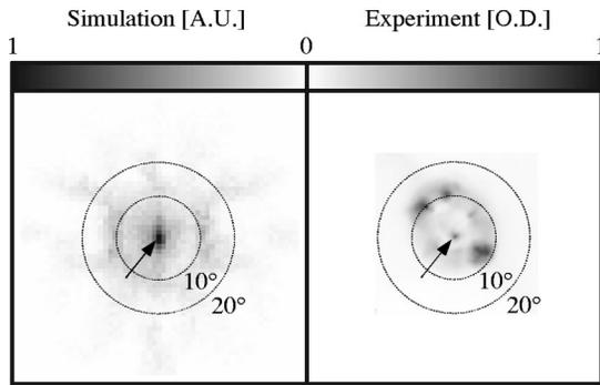
FIG. 3. 3D PIC simulation: angular distribution with respect to the laser axis of the electrons emitted forward (left), to be compared with the radiochromic film data (right). The two arrows indicate the energetic electron beam in the two cases.
