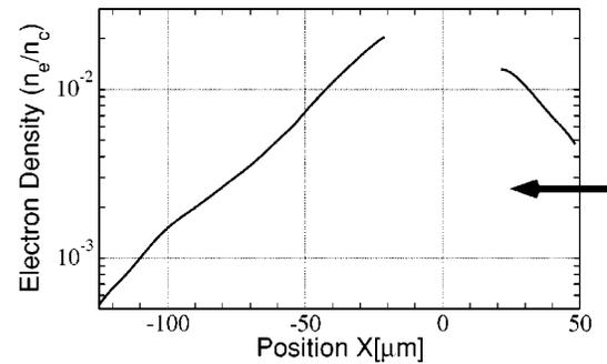
FIG. 1. Longitudinal electron density profile of the plasma as inferred from an interferogram taken 50 ps before the arrival of the 35 fs pulse. The arrow shows the direction of the laser pulse propagation. The  $X=0$  position indicates the initial position of the foil target. The critical density  $n_c$  refers to  $\lambda=815 \text{ nm}$ .
