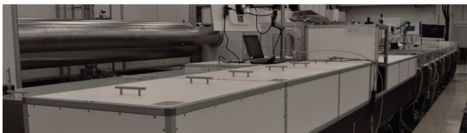
Fig. 29.9. The L4 “Aton” laser system is under development now at ELI-Beamlines (2 kJ, 1 shot/min) (image courtesy of ELI Beamlines).
