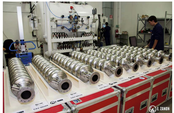
Fig. 1. A set of pre-series XFEL cavities at the company E. Zanon.
