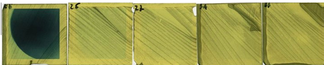
Fig. 3. Impressed EBT3 radio-chromic film.
