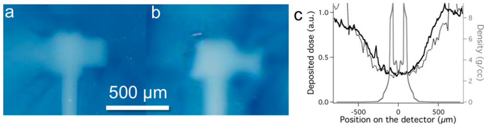
Figure 3. Proton radiography images of the compressed cylinder (a) without compression and (b) with compression at \tau = 1.2 ns, and a 0.1 \text{ g cm}^{-3} initial plastic foam inside the cylinder. (c) Experimental (dark solid line) and simulated (dotted line) example profiles. The grey line is the corresponding density profile. The cylinder is initially filled with 0.1 \text{ g cm}^{-3} plastic foam for all these cases.
