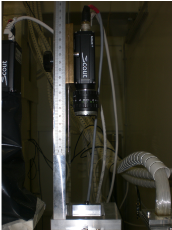
Figure 6: Left: Picture of a camera mounted on the metal support pointing to the fiber matrix. Right: Picture of the LabView Panel of the VI used for identifying the 64 channels from a calibration image obtained with the digital camera.
