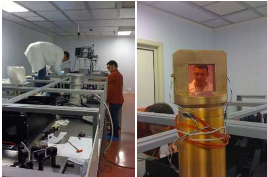
Figure 1: Main amplifier pumps alignment, cryo amplifier installation.
