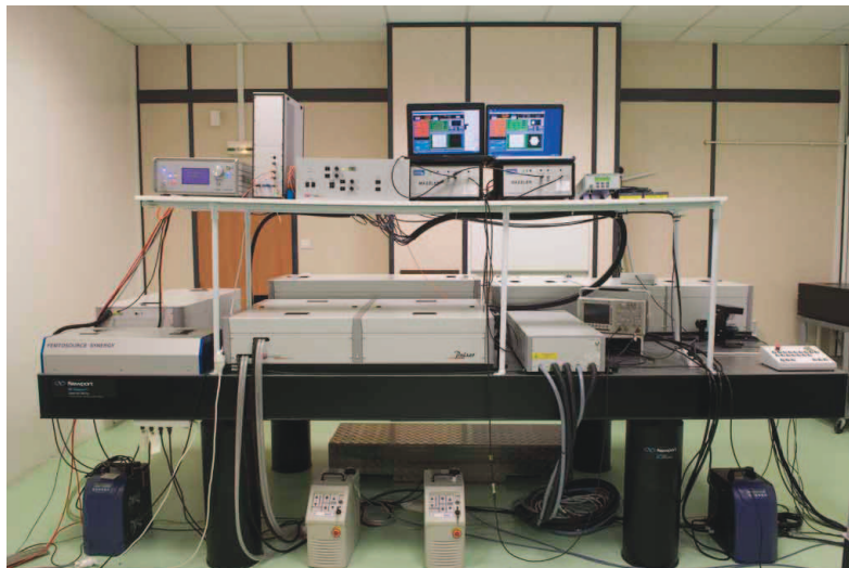
Figure 1: Front end of the FLAME laser system assembled for testing at the factory. The front end includes the advanced system for contrast enhancement and DAZZLER-MAZZLER combination for bandwidth and pulse duration optimisation.
