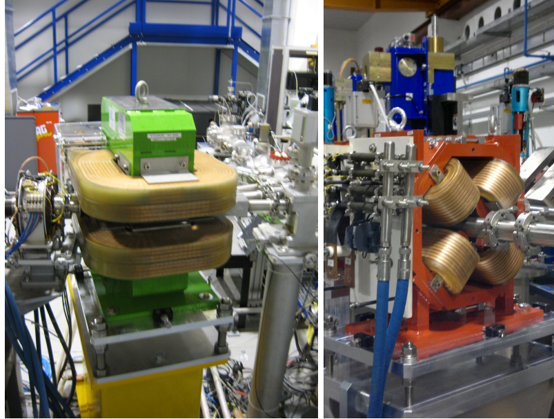
Figure 12: Dipole (left) and Quadrupole (right) magnets of the PlasmonX electron beamlines.
