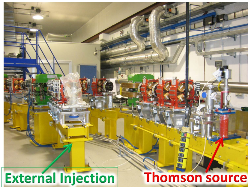
Figure 13: Final part of the Plasmonx electron beam transfer lines up to the two interaction points.
